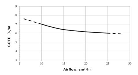
Highest possible SOTE at high airflow rates tested per ASCE standard.
