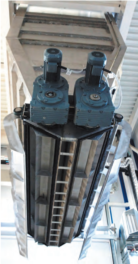
SILOS for accumulating 48 m 3 of cake with a paddle turner-dispenser and bucket gates.
